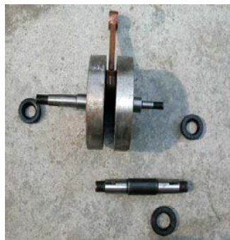
GGG crank and oil seals shown for clarification purpose
