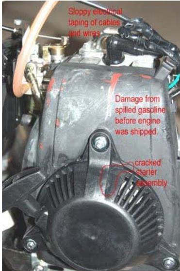
Condition of engine when removed from packing carton: Wires sloppily and loosely gathered with electrical tape, a large crack in the pull-starter housing, and the large plastic magneto cover stripped and corroded by gasoline.
