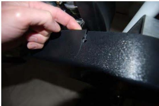
The very heavy-duty black plastic housing that encloses the Q-Matic gearbox is missing one of its four mounting fasteners, and there is a crack radiating the full width of the housing.
