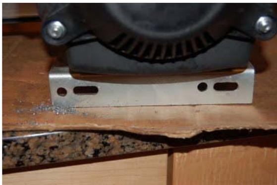
The adjustable-length holes in the mounting plate on the bottom of the engine wouldn't match up with the threaded holes in the frame-mounted motor mounts. So I had to drill two new holes on each side of the mounting plate, and then extend the adjustment holes to the new holes with a Dremel.
