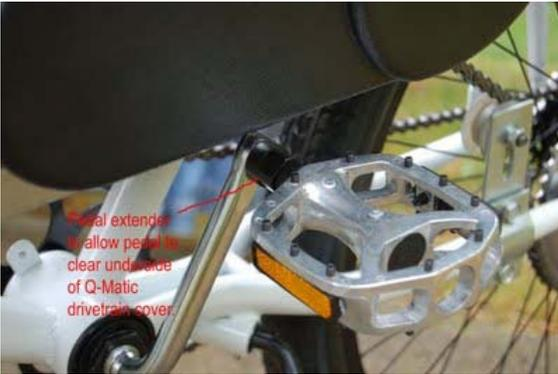
The left-side pedal wouldn't clear the underside of the gearbox housing (and the end of the crank arm just clears it). So I had to research this problem for a solution, seek out a source for pedal extenders, and purchase them online.
