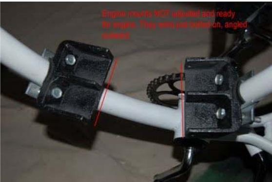
The motor mounts on the frame should have been adjusted to exactly the correct position to accept the engine's mounting plate, but the engine had apparently never been mounted for testing of the bike before shipping. This photo shows the motor mounts as they looked when the bike was unpacked: angled outwards to the left and fully tightened!
